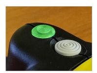
LED provides PASS/FAIL indication on the probe for fast verification of connector status.
